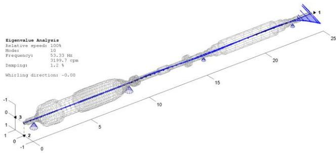
**Figure 4: 3D mode shape of the bending critical of the shaft end**
