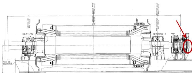
**Figure 6: Chosen balancing plane of the generator shaft end**
