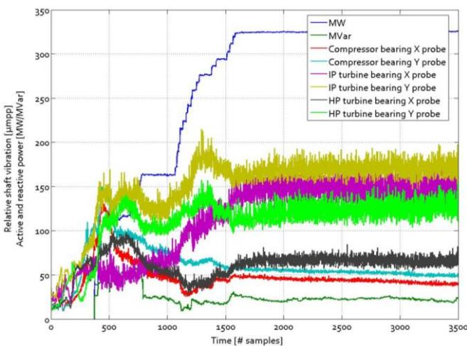
Figure 12: Relative shaft vibration amplitudes for different load conditions
