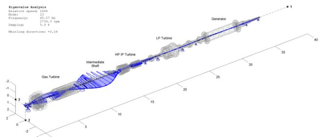
Figure 15: Mode shape of the 3<sup>rd</sup> horizontal bending mode of the GT
