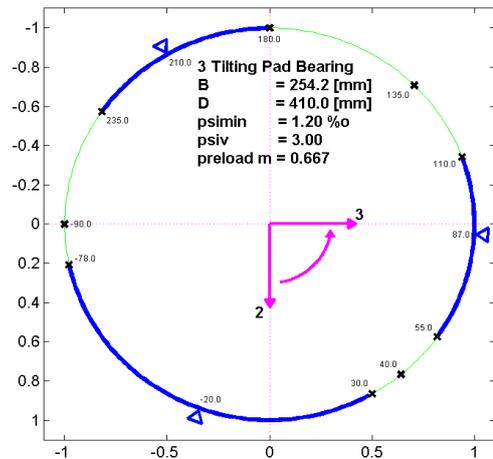
**Figure 17: HP/IP bearing geometry**
