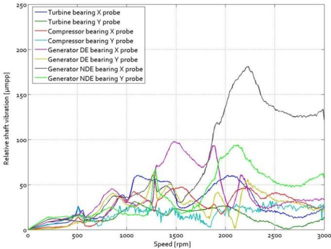
**Figure 9: Relative shaft vibration amplitudes after balancing**
