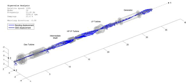
**Figure 16: Mode shape of the 2<sup>nd</sup> horizontal bending mode of the IP/HP turbine**
