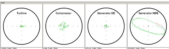
**Figure 5: Direct orbit plots at 2980rpm**
