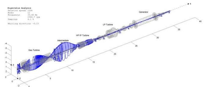
Figure 14: Mode shape of the 3<sup>rd</sup> vertical bending mode of the GT
