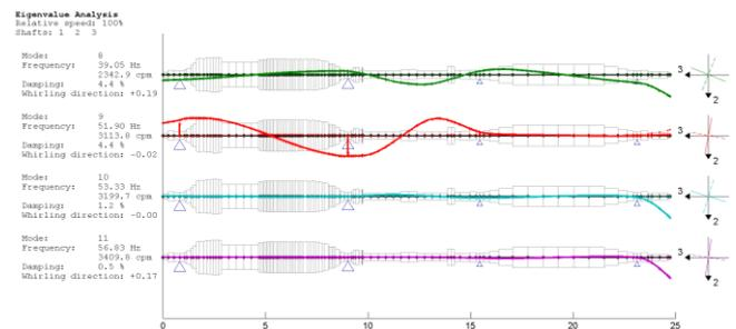
Figure 3: Eigenvalue analysis of the shaft line
