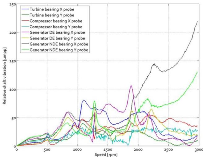
Figure 1: Relative shaft vibration amplitudes during startup
