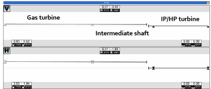
Figure 13: "Hot" alignment condition of the GT - IP/HP
