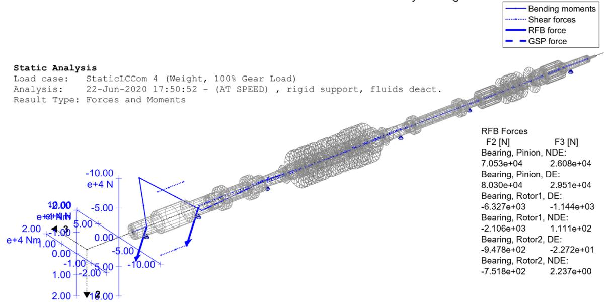
Fig. 1.5: Forces in the shaft train with many bearings, results with rigid bearings
