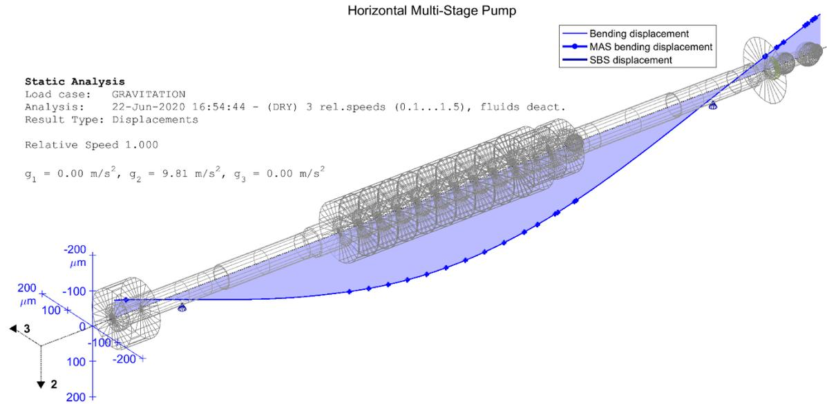
Fig. 1.7: Static displacements without fluids (dry), 100% speed
