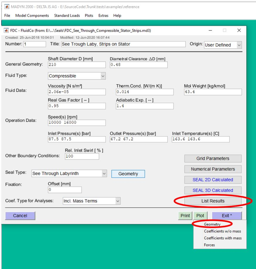
Fig. 3.1: GUI for user defined FDC with additional item for the geometry
