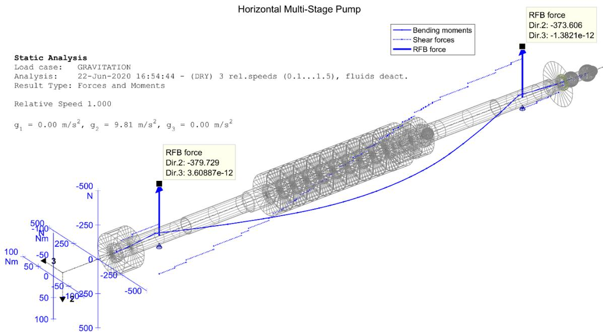
Fig. 1.8: Static forces without fluids (dry), 100% speed
