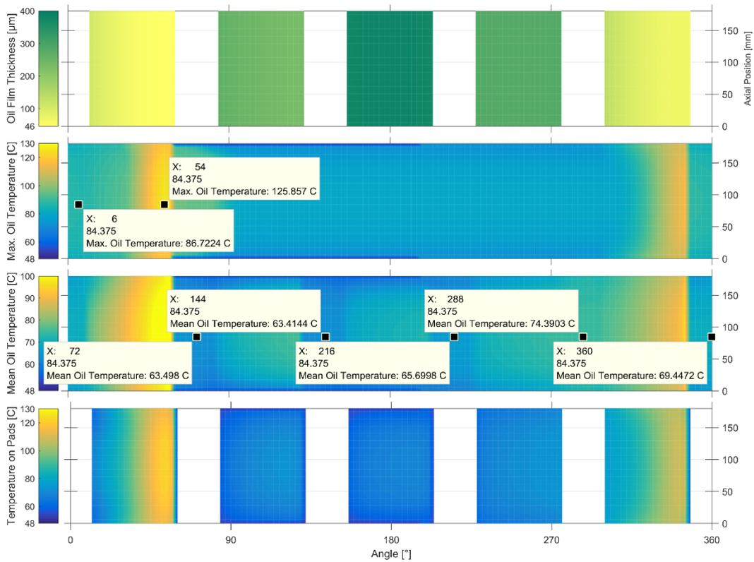
Fig.5.2: Minimum oil film thickness and temperatures
