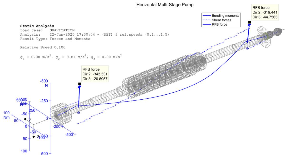
Fig. 1.10: Static forces with fluids (wet), 10% speed
