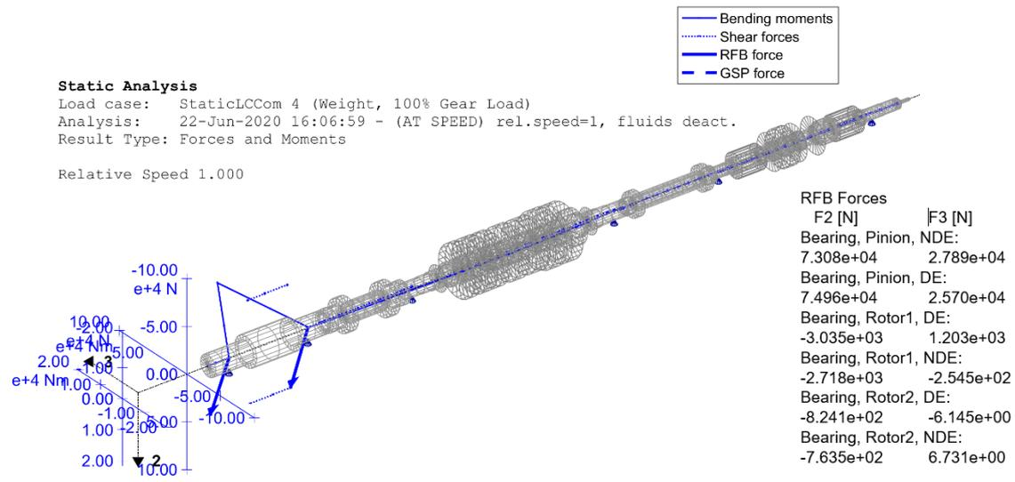
Fig. 1.3: Forces in the shaft train with many bearings, results with oil film
