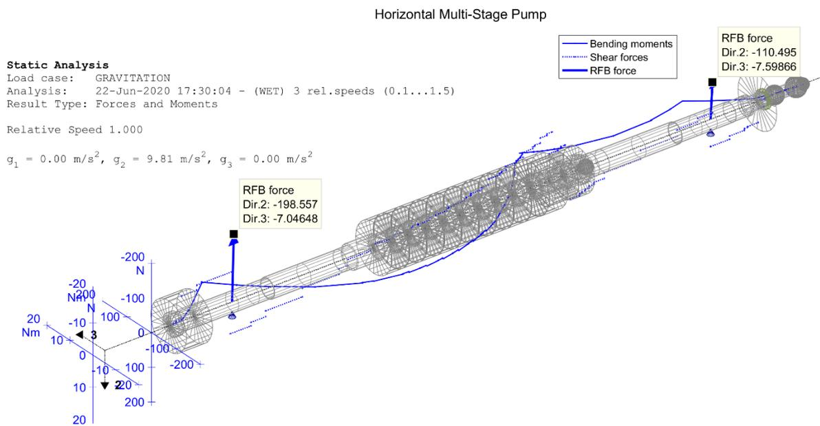
Fig. 1.12: Static displacements with fluids (wet), 100% speed
