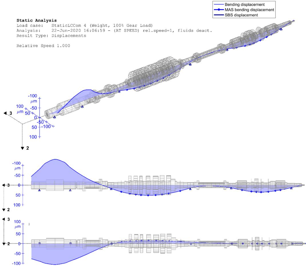
Fig. 1.2: Displacement of the shaft train with many bearings, results with oil film
