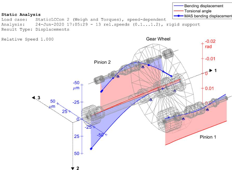
Fig. 2.3: Static deformation due to weight and torques at 10% and 100% speed
