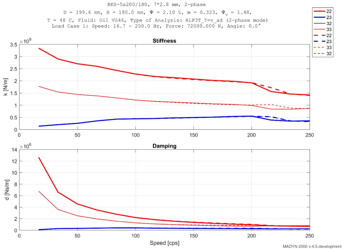
Fig. 5.4 Rotordynamic coefficients calculated in versions 4.5 and 4.4 (dashed lines)
