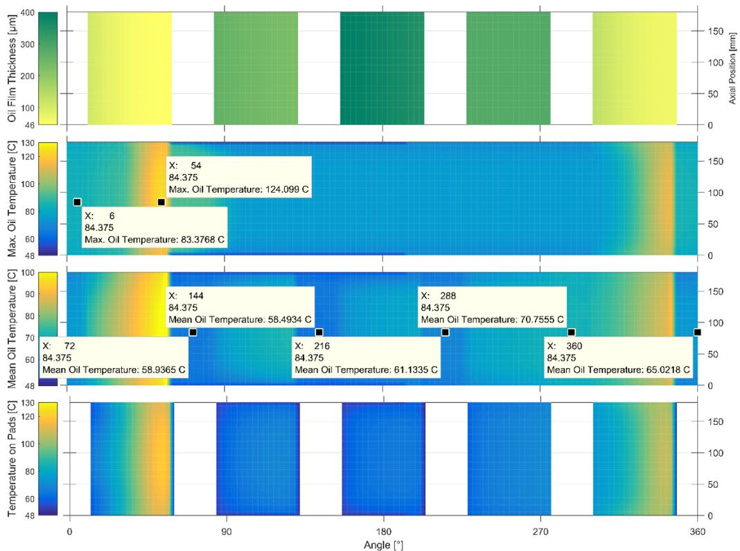
Fig.5.3: Minimum oil film thickness and temperatures calculated with version 4.4
