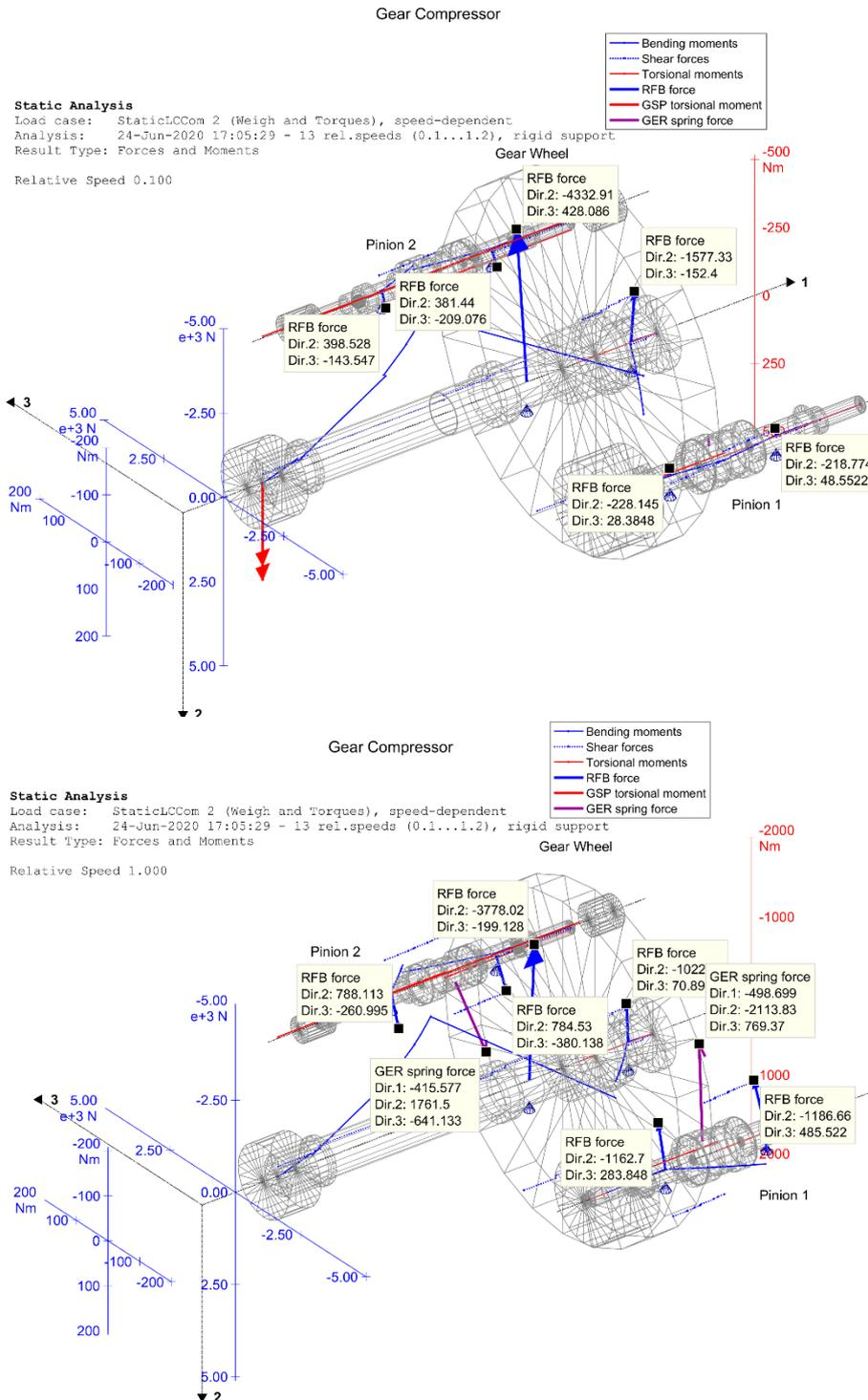
Fig. 2.4: Static forces due to weight and torques at 10% and 100% speed
