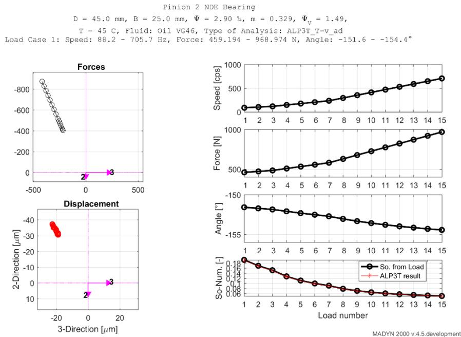
Fig. 2.7: Load case variants created for the pinion 2 bearings in the Campbell diagram analysis
