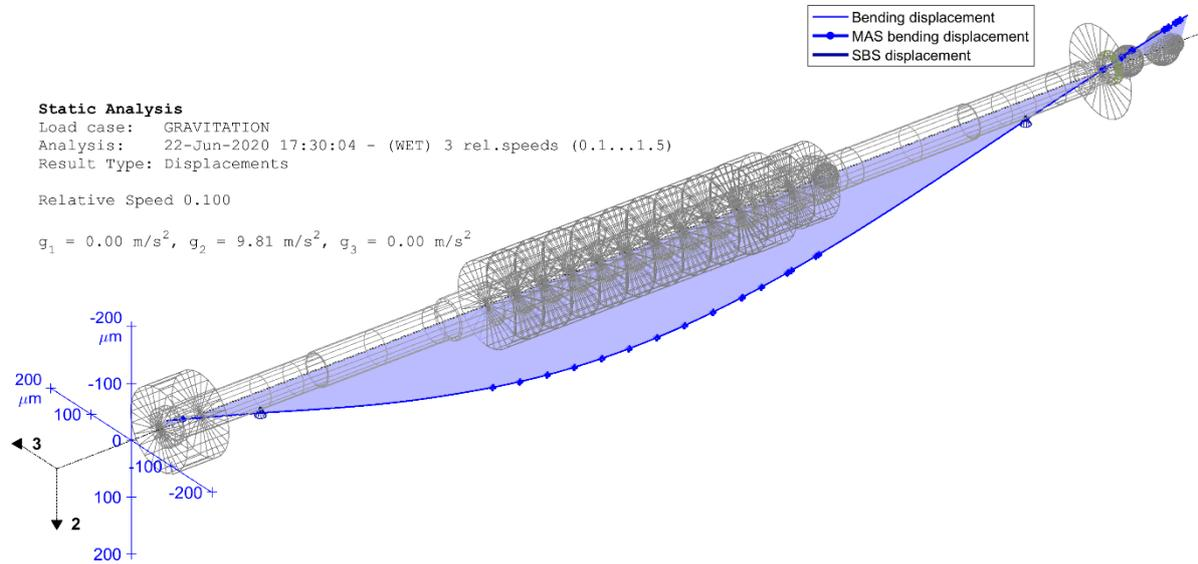
Fig. 1.9: Static displacements with fluids (wet), 10% speed
