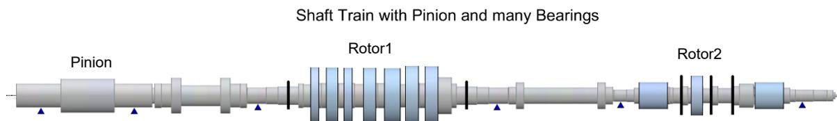
Fig. 1.1: Shaft train with a pinion and many bearings
