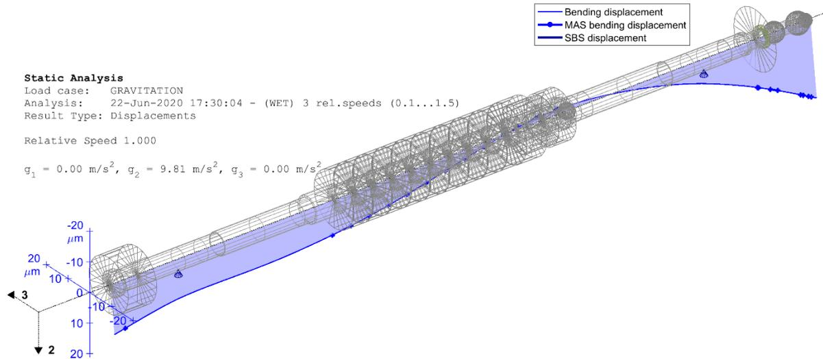
Fig. 1.11: Static displacements with fluids (wet), 100% speed
