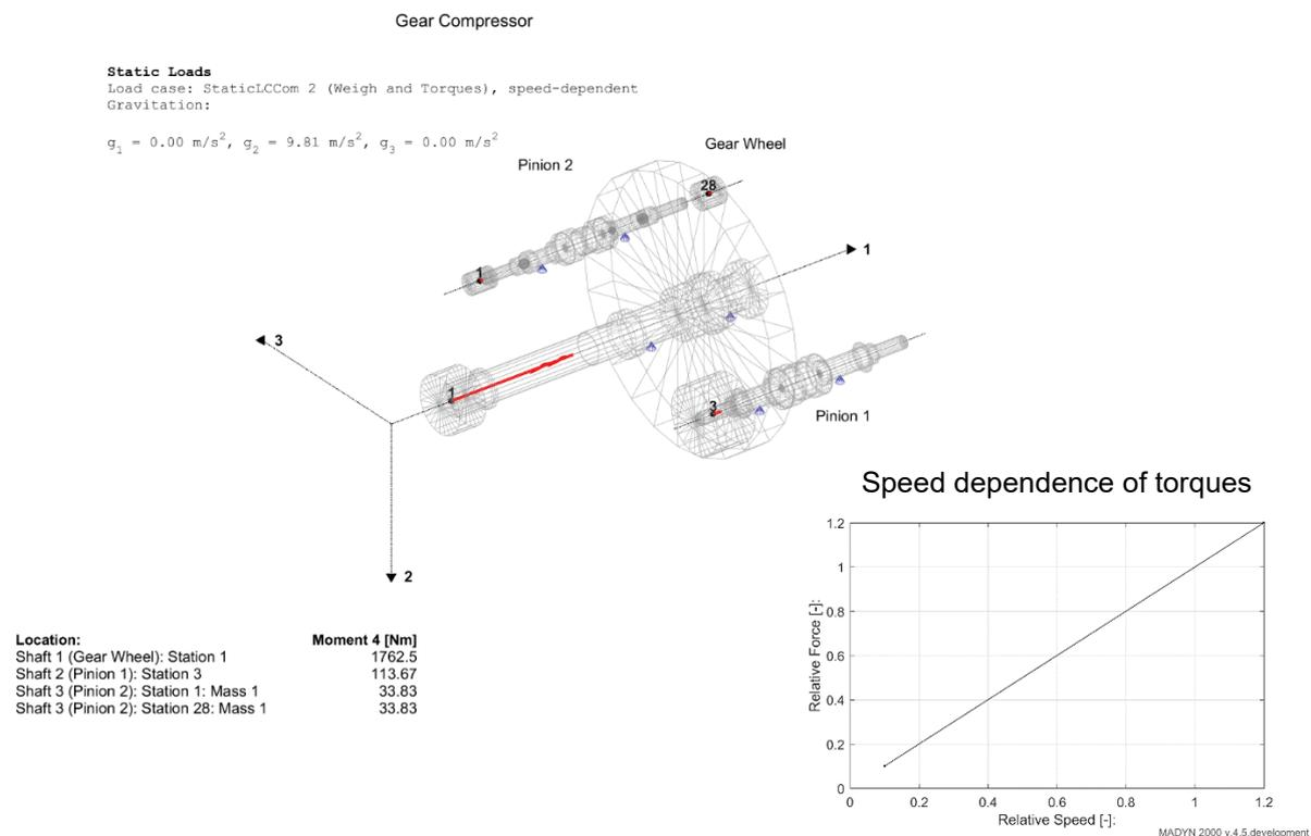
Fig. 2.2: Speed dependent driving torque and counter torques
