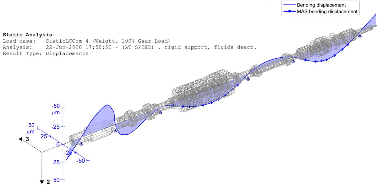
Fig. 1.4: Displacement of the shaft train with many bearings, results with rigid bearings
