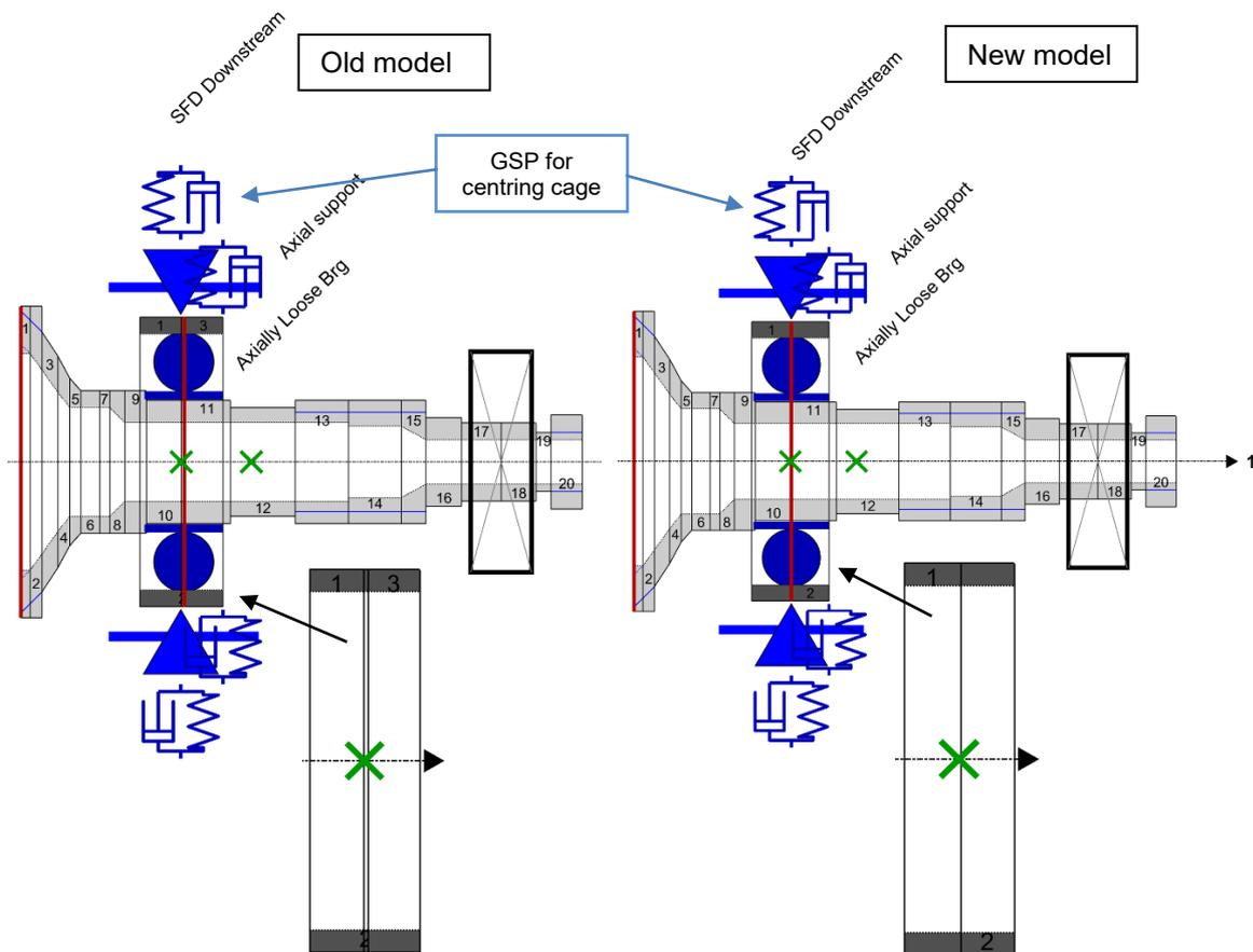
Fig. 4.3: Downstream shaft end with rolling element bearing and squeeze film damper
