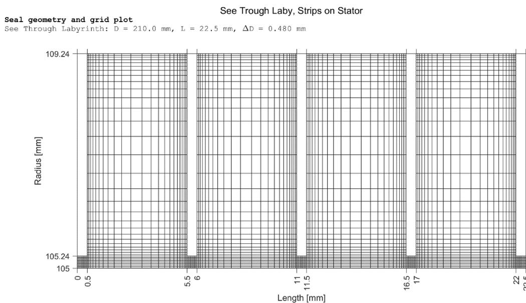
Fig. 3.2: Seal geometry plot
