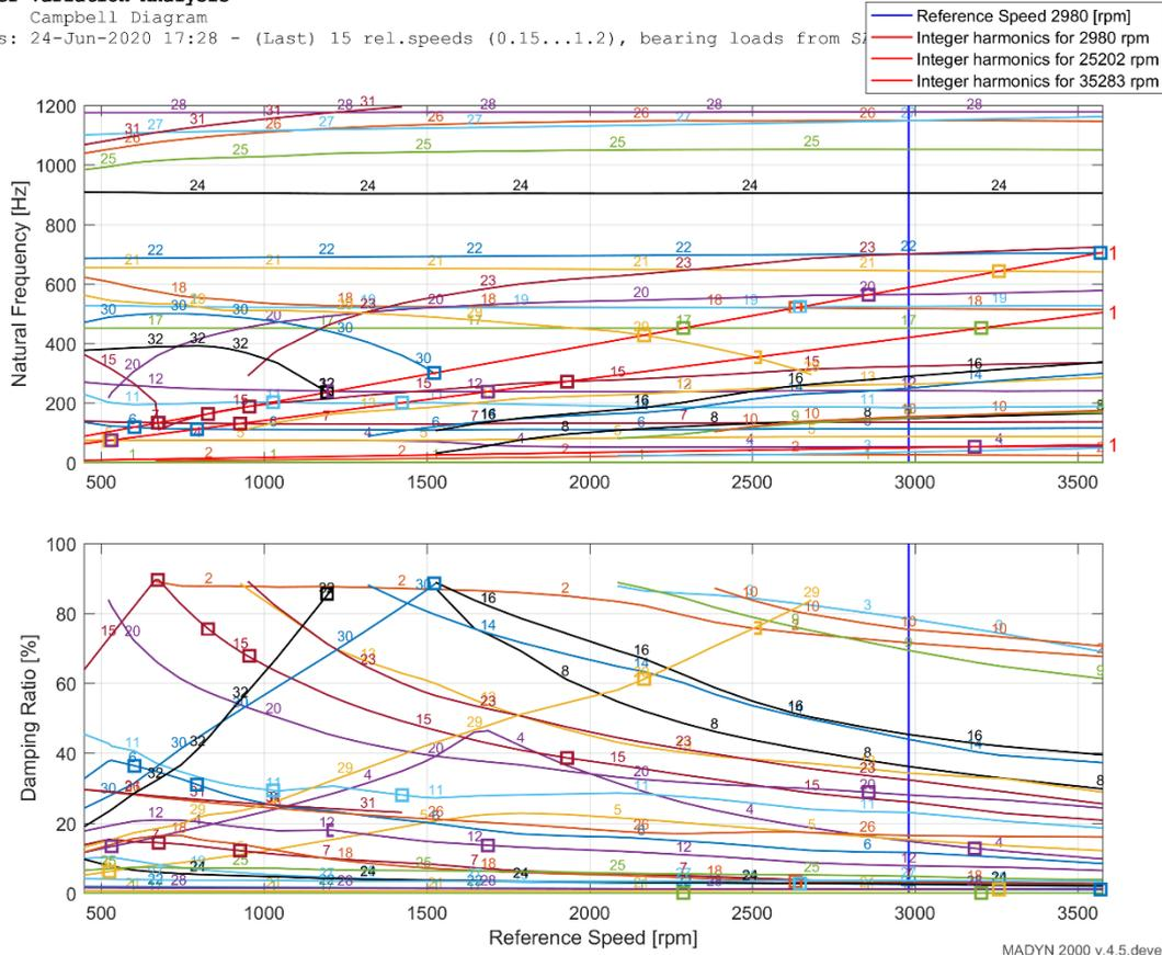
Fig. 2.9: Campbell diagram of the lateral torsional coupled system of a gear compressor
