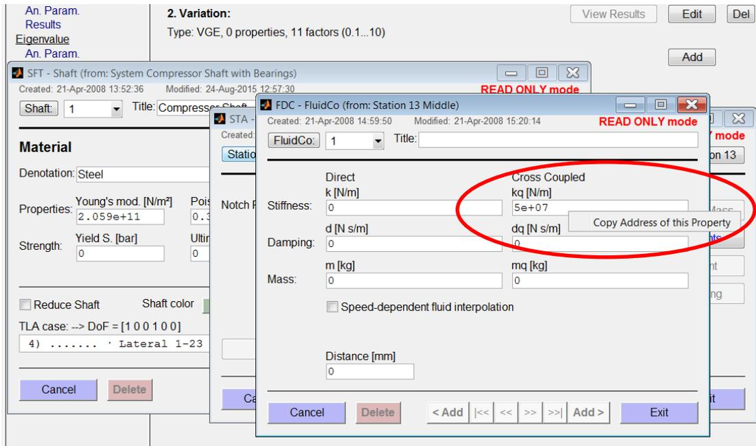
Fig. 2.2: Copying the address of the fluid coefficient  $k_q$ .
