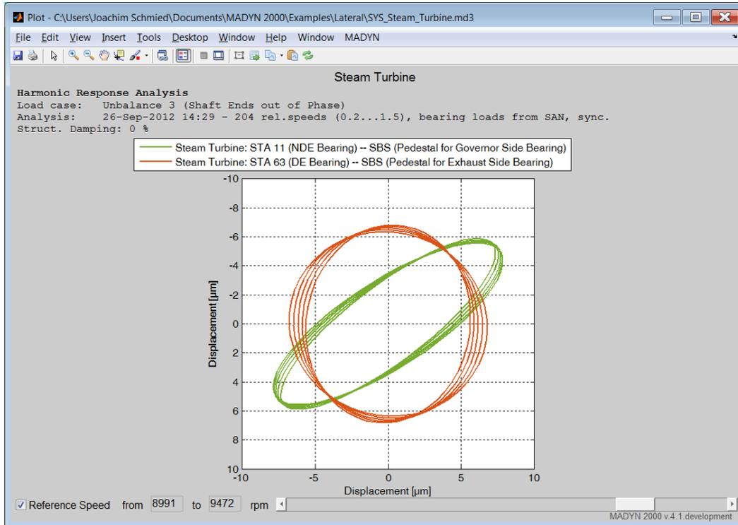
Fig. 3.5: Orbit plot with scroll bar to define parameter range
