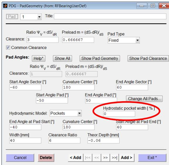
Fig. 5.5: Closing the hydrostatic pocket before the 1<sup>st</sup> pad by setting the width to zero
