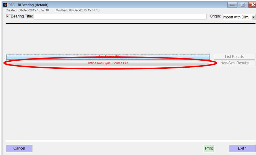
Fig. 7.1: GUI for imported dimensioned data with button to import non-synchronous bearing characteristics
