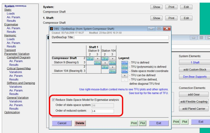
Fig. 4.1: DBS GUI with new check box for the state space reduction and an edit filed to define the order
