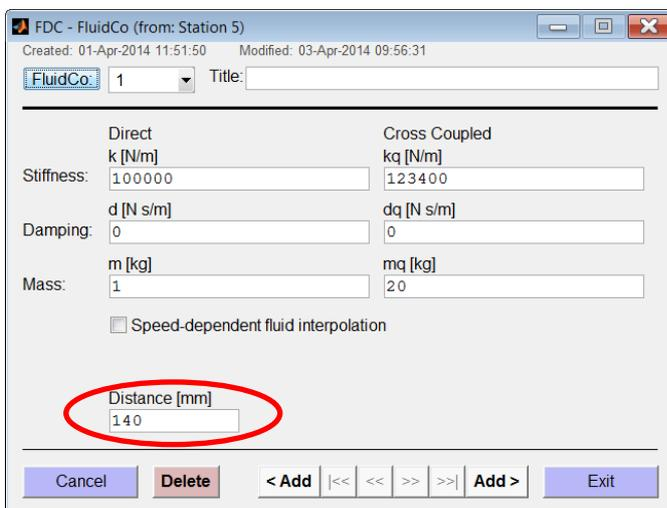
Fig. 8.1: GUI for fluids with the edit field to define a distance or offset
