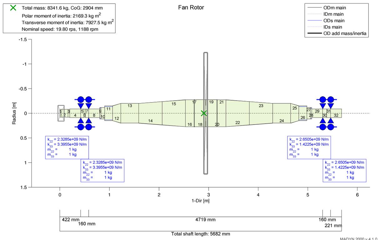
Fig. 5.7: Example of a sensitive fluid film bearing arrangement regarding static analysis
