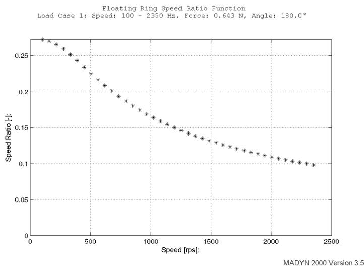
Figure 5.4: Ring speed ratio as a function of speed
