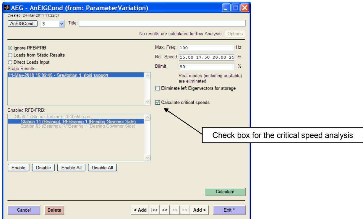
Figure 3.1: Campbell diagram analysis GUI with check box for critical speed analysis
