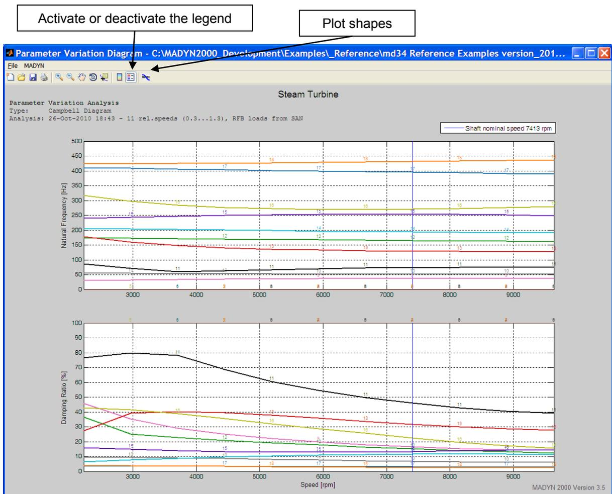
Figure 10.1: Explanation of new icons for plots for the example of Campbell diagrams
