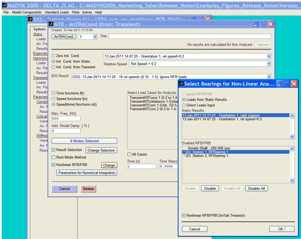
Figure 4.2: Transient analysis GUI with Bearing GUI for nonlinear bearings
