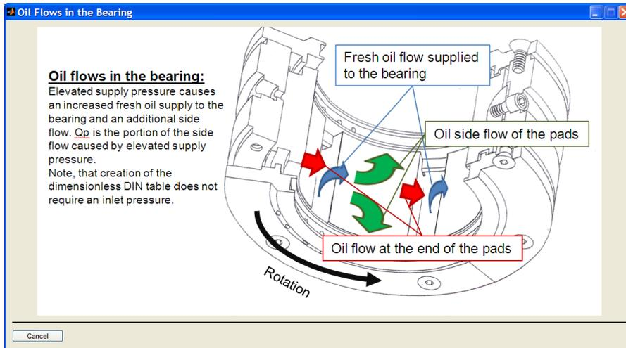
Figure 6.2: Oil flows in the bearing for the explanation of  $Q_p$
