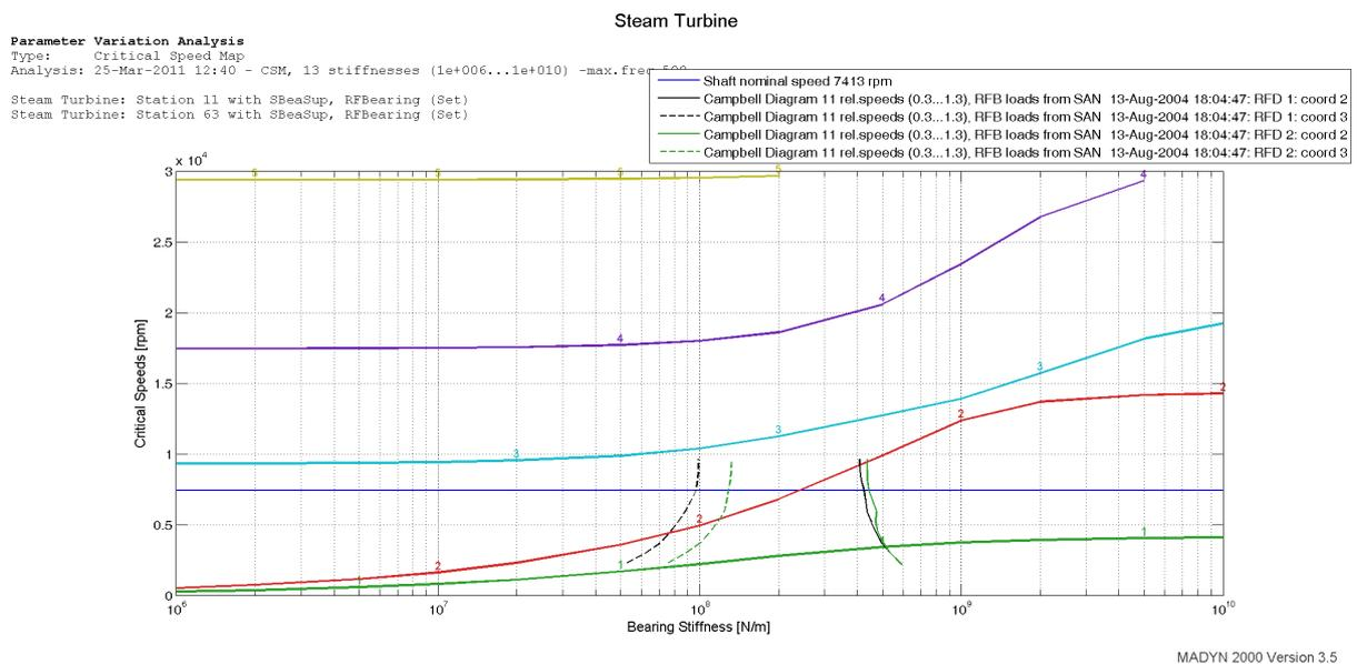
Figure 8.2: Critical speed map with fluid film bearing stiffnesses from a Campbell diagram
