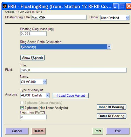
Figure 5.3: FRB GUI with “Show f(Speed)” button in case of speed dependent ring speed ratio
