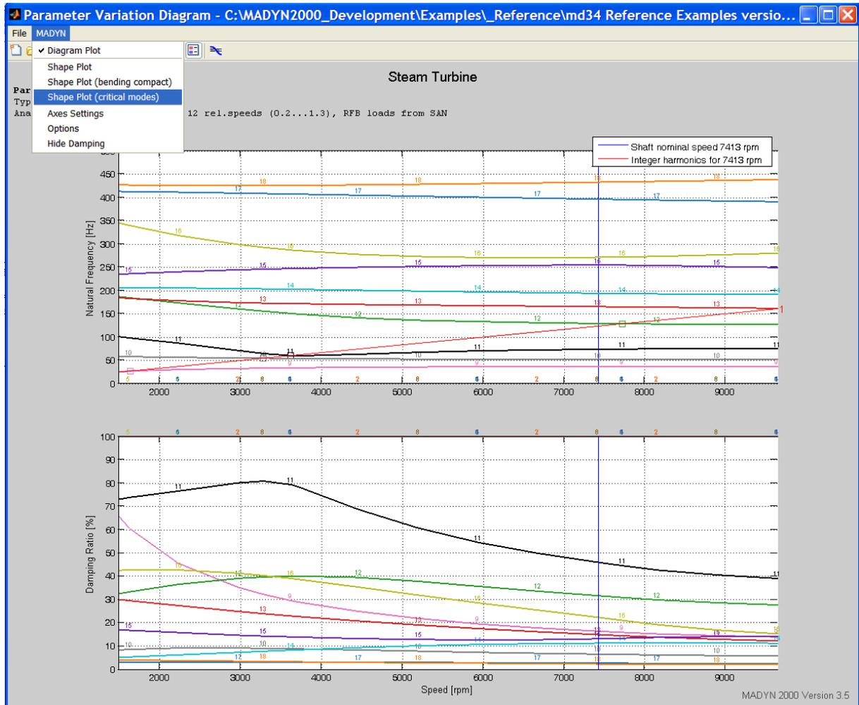
Figure 3.2: Campbell diagram with Critical speeds and menu to plot the associated mode shapes
