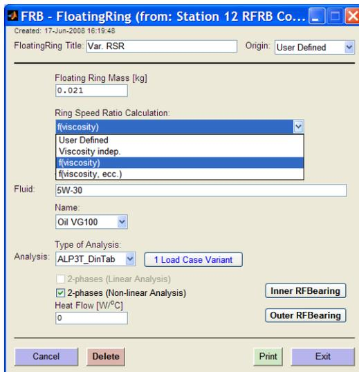
Figure 5.2: Additional options to define the ring speeds for "DinTab" and "c\_ad"
