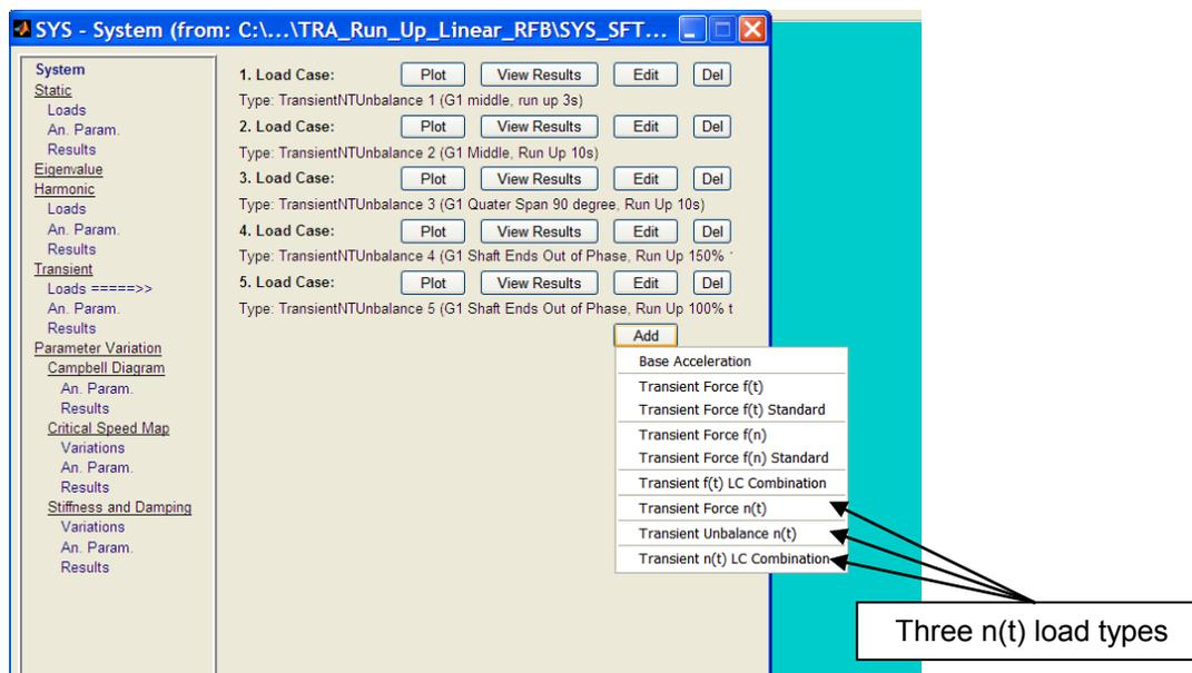
Figure 1.1: Menu to create  $n(t)$  transient loads
