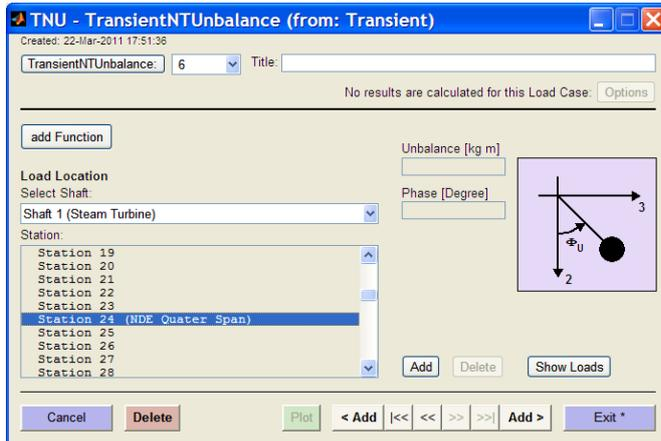
Figure 1.2: GUI for Unbalance n(t) loads
