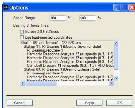
Figur 8.1: GUI to select bearing stiffnesses to be drawn in the Critical Speed Map
