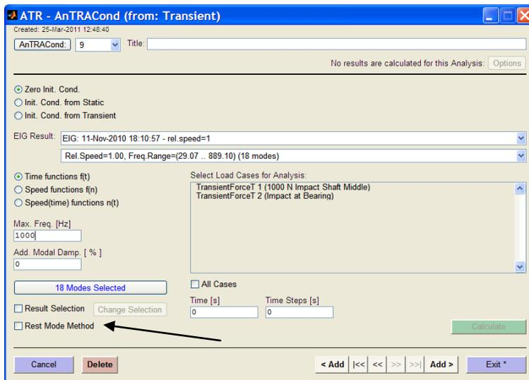
Figure 9.1: Transient analysis GUI with check box to apply the “Rest Mode Method”
