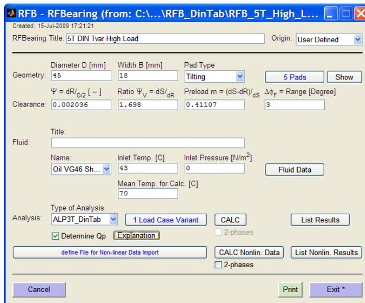
Figur 6.1: RFB GUI for “DinTab” analysis with check box “Determine Qp”
