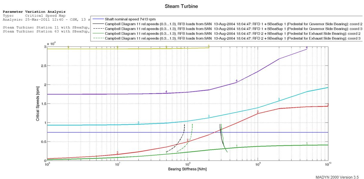
Figure 8.3: Critical speed map with fluid film bearing stiffnesses from a Campbell diagram including the support stiffness
