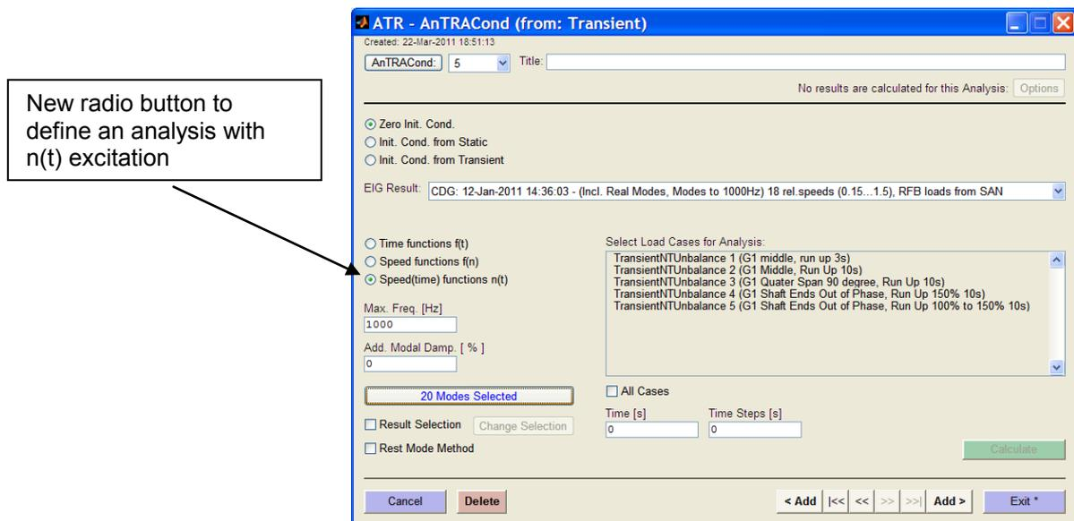
Figure 1.6: Transient analysis GUI with  $n(t)$  selection
