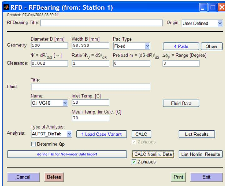
Figure 4.1: RFB GUI for analysis type ALP3T\_DinTab and nonlinear characteristics with 2-phase
