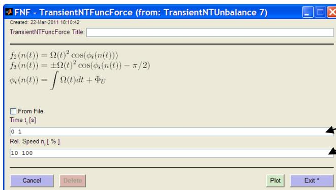
Figure 1.4: GUI for the n(t) unbalance excitation function
