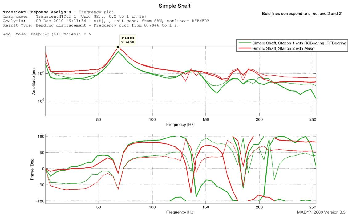
Figure 2.4: Spectrum of the time history in figure 1.10 in the unstable range (0.8s to 1s)
