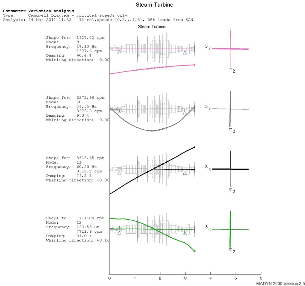
Figure 3.3: Mode shapes in the critical speeds
