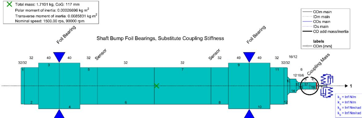
Fig.2: Rotor model on foil bearings
