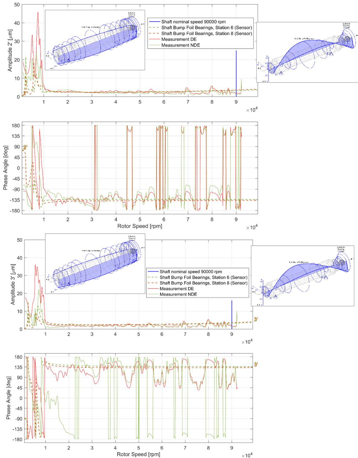
Fig. 8: Measured and calculated unbalance response in 2' and 3' direction (45° to vertical) with shapes at 40'000rpm and 90'000rpm.
