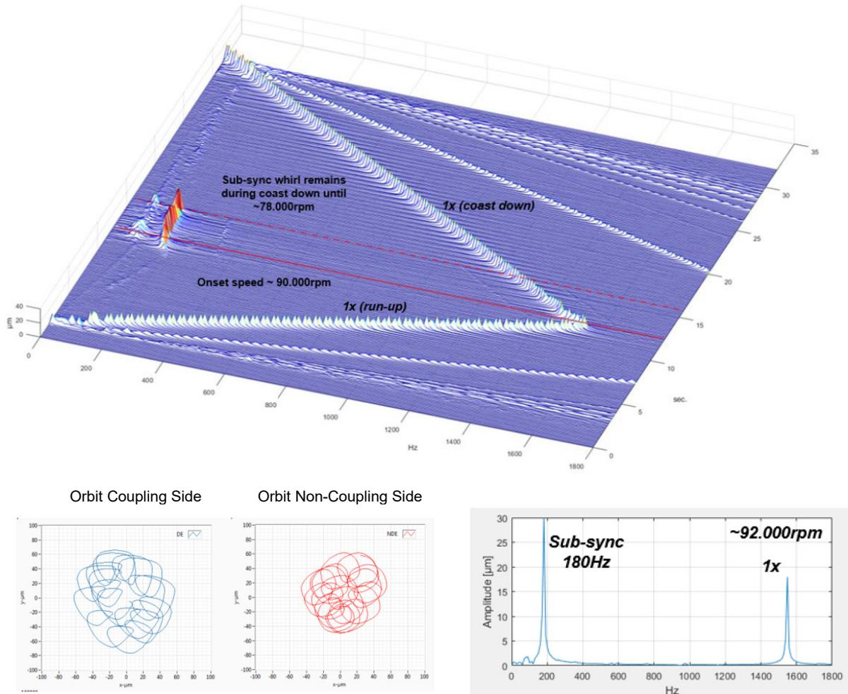
Fig. 6: Measured Waterfall plot of the test, spectrum and orbits at 92'000rpm (from /2/)
