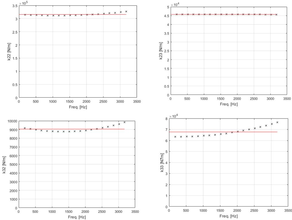
Fig. 3: Calculated (black cross) and adapted (red line) frequency dependent stiffness coefficients
