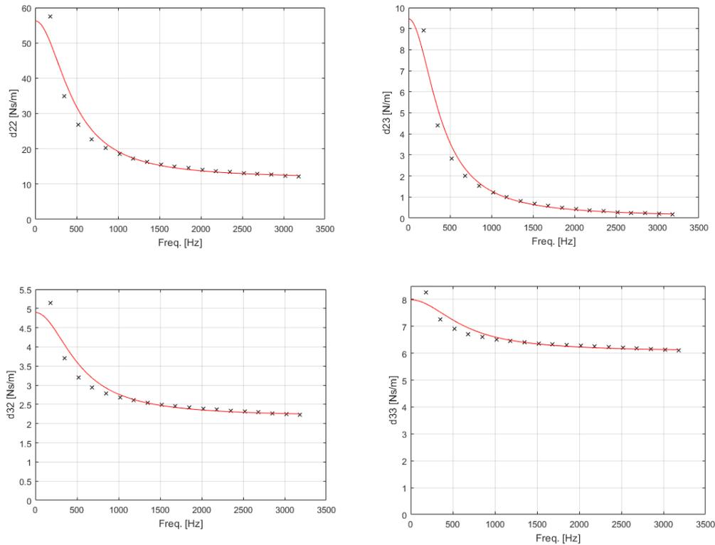
Fig. 4: Calculated (black cross) and adapted (red line) frequency dependent damping coefficients
