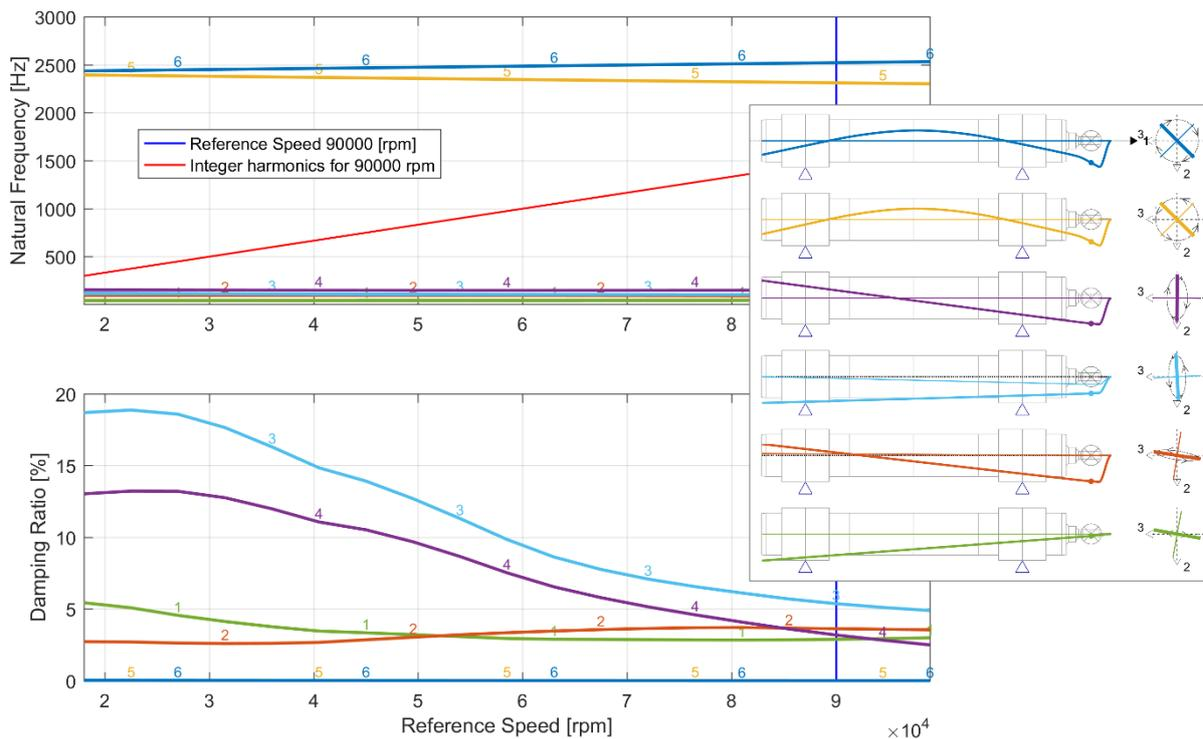
Fig. 5: Campbell diagram with mode shapes at 90'000rpm
