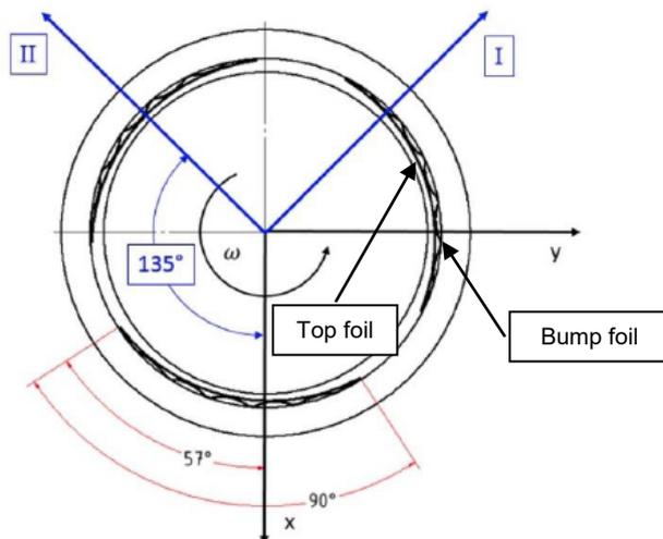
Fig.1: Example of a foil bearing (from /2/).
