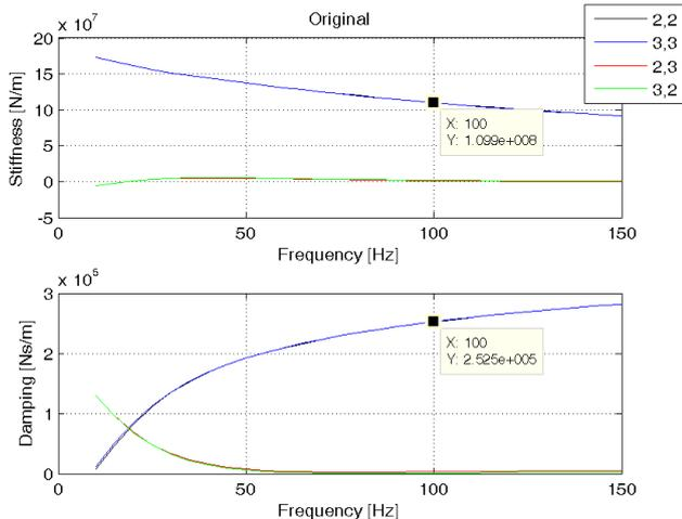
Fig.5 Stiffness and damping coefficients at 6000rpm, 4-tilting pad bearing 55% offset
