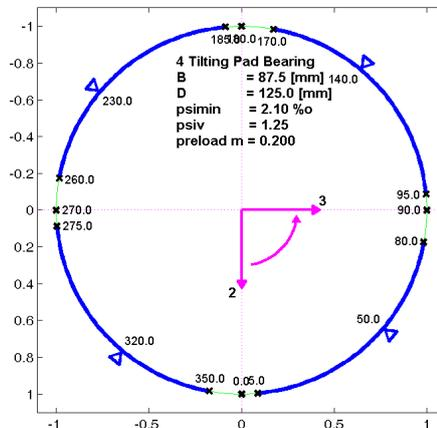
Fig.3 4-tilting pad bearing, 60% offset
