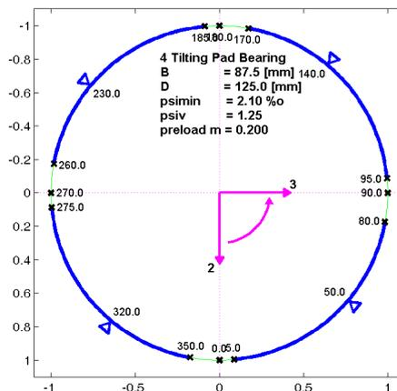
Fig.3 4-tilting pad bearing, 60% offset
