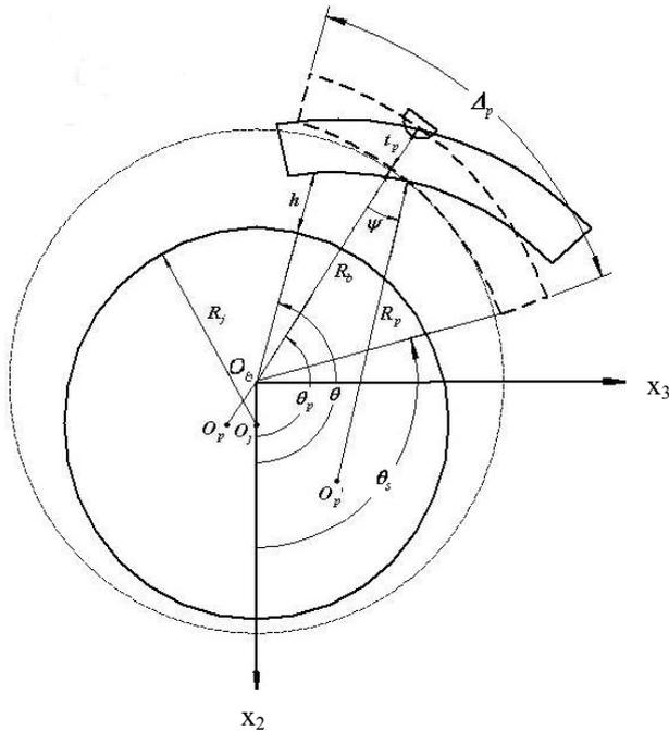
Fig.1 Pad geometry of a tilting pad bearing
