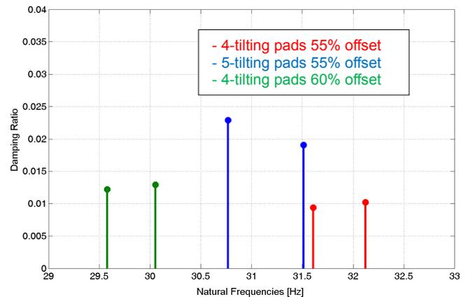
**Fig.10 Eigenvalues of the 1<sup>st</sup> mode, extended model**
