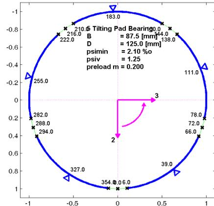
Fig.2 5-tilting pad bearing, 55% offset
