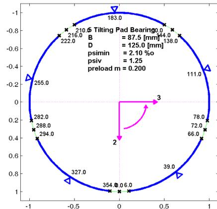
Fig.2 5-tilting pad bearing, 55% offset
