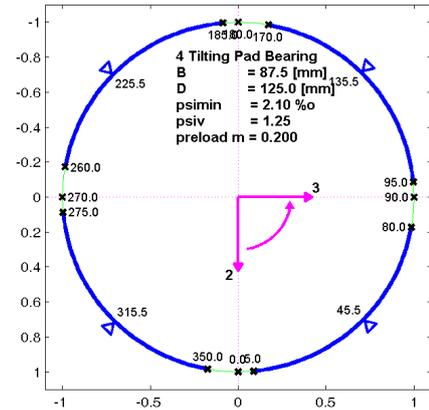
Fig.1 4-tilting pad bearing, 55% offset
