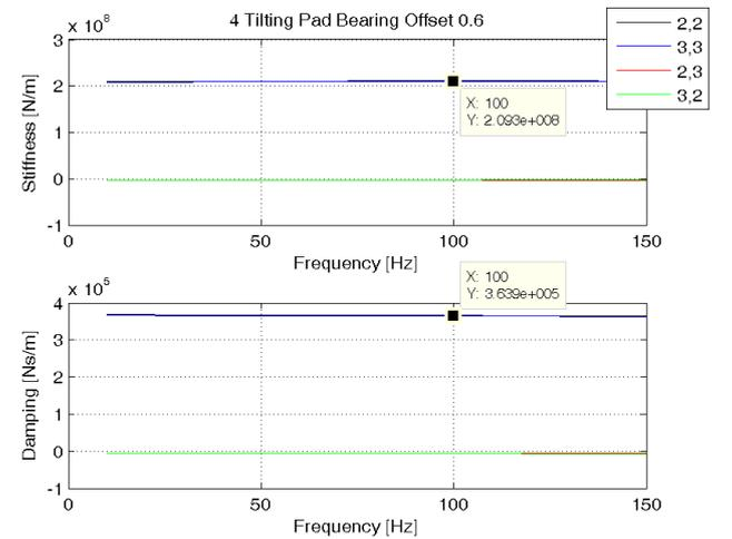
Fig.7 Stiffness and damping coefficients at 6000rpm, 5-tilting pad bearing 60% offset
