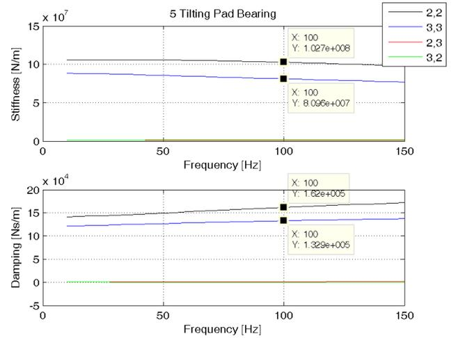
Fig.6 Stiffness and damping coefficients at 6000rpm, 5-tilting pad bearing 55% offset
