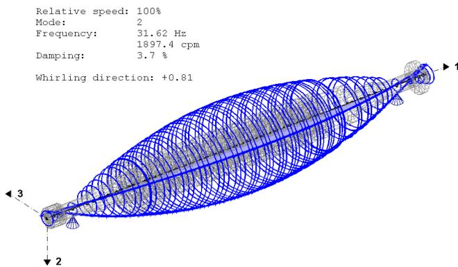
**Fig.8 First natural mode with synchronous coefficients, 4-tilting pad bearings, 55% offset**
