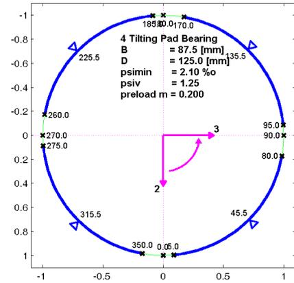
Fig.1 4-tilting pad bearing, 55% offset
