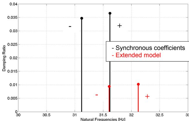
**Fig.9 Eigenvalues of the 1<sup>st</sup> mode, 4-tilting pad bearing, 55% offset**
