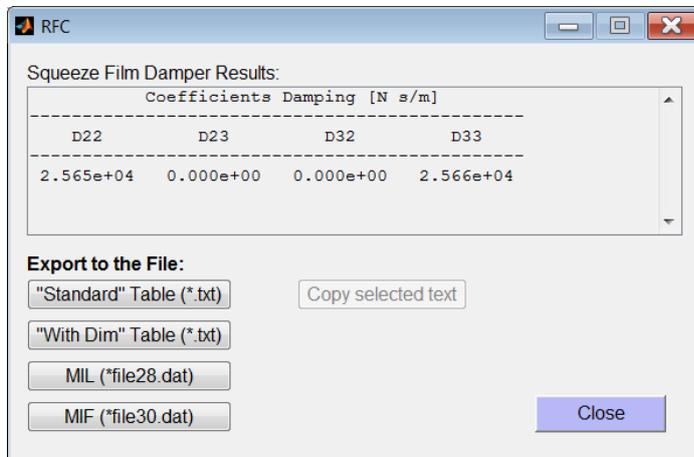
Fig. 5.2: Linear characteristics of a squeeze film damper (window available from "List Results")
