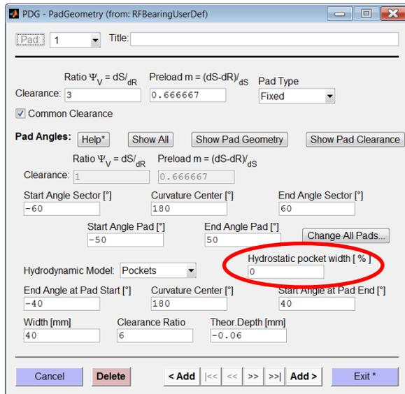
Fig. 5.5: Closing the hydrostatic pocket before the 1<sup>st</sup> pad by setting the width to zero
