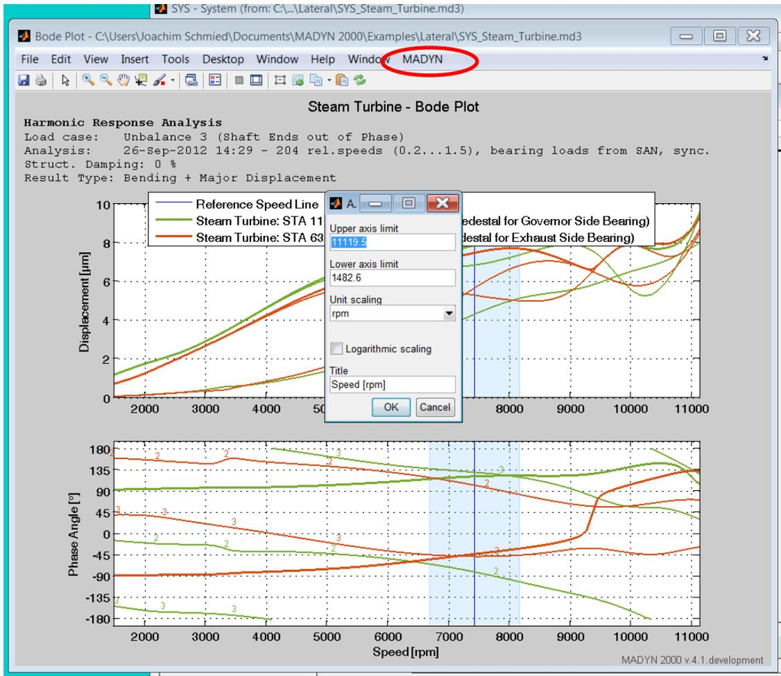
Fig. 3.4: Axes configuration and MADYN menu in plot window
