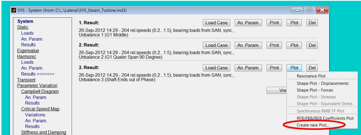
Fig. 3.1: Menu with item to create configurable plots from plot button in system explorer
