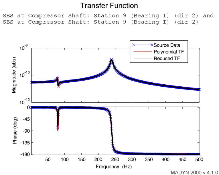
Fig. 4.3: Transfer function plot for a single support for all available forms
