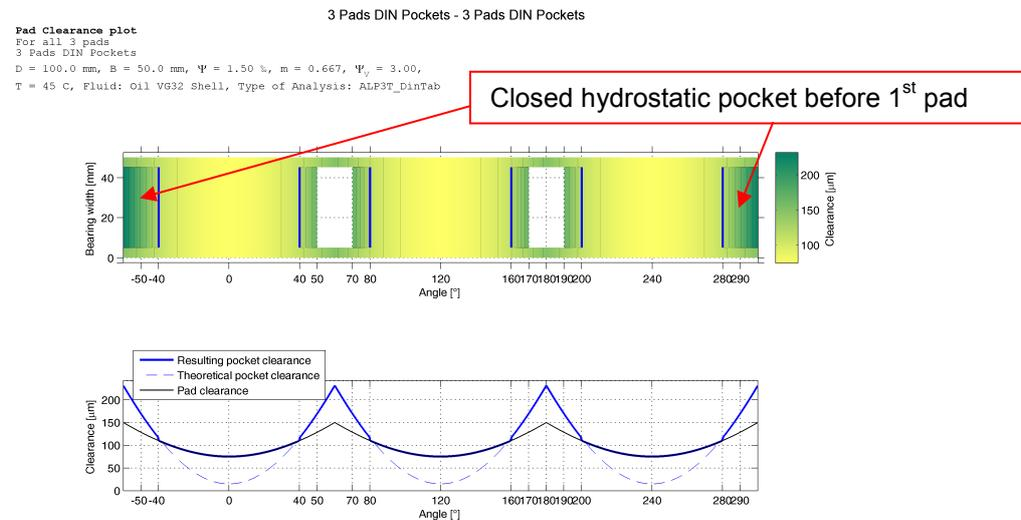
Fig. 5.6: Bearing clearance plot with closed hydrostatic pocket before the 1<sup>st</sup> pad
