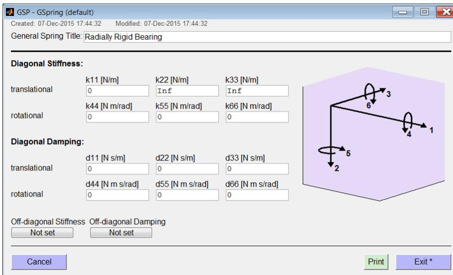
Fig. 9.1: GSP GUI with definition of a rigid radial support
