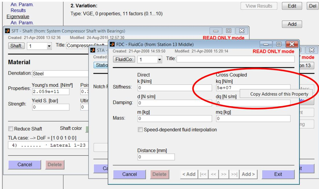
Fig. 2.2: Copying the address of the fluid coefficient  $k_q$ .
