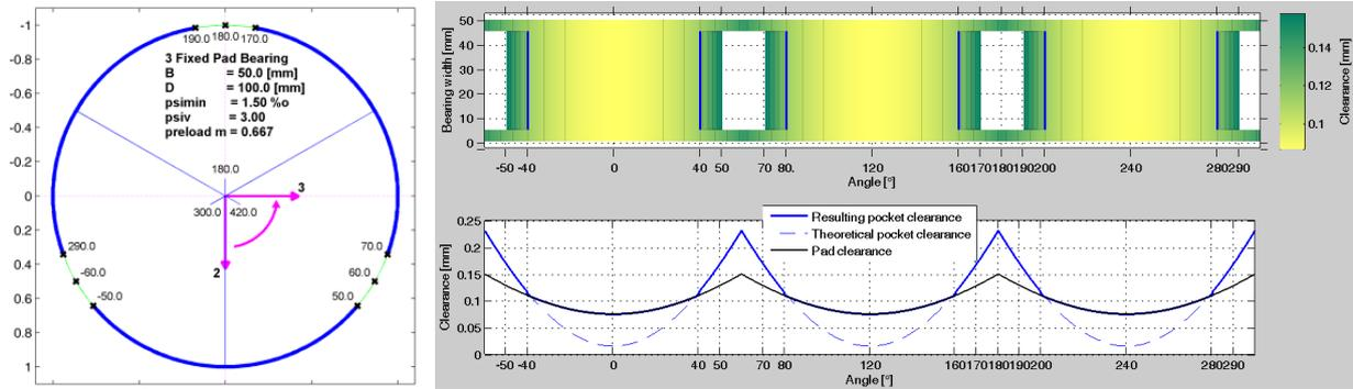
Fig. 5.4: Hydrostatic pockets between 50° to 70°, 170° to 190° and 290° to -50°
