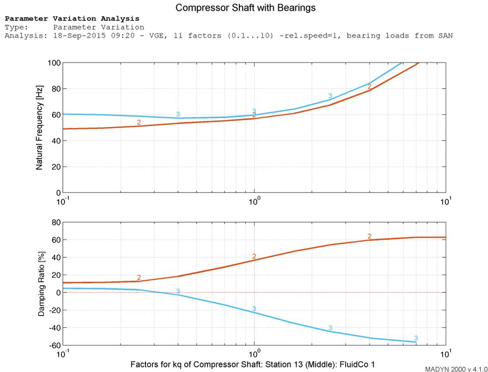
Fig. 2.4: Diagram of the eigenvalues for the variation of a fluid cross coupling coefficient
