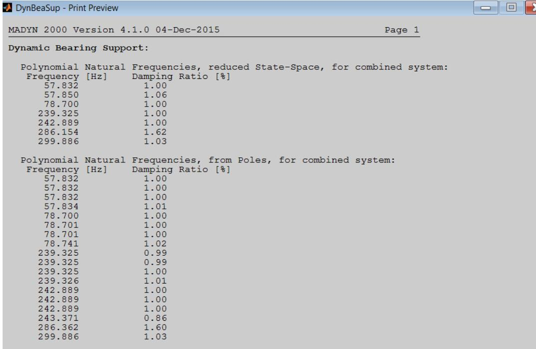
Fig. 4.2: Print of the eigenvalues of the DBS state space system, reduced and original order
